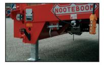
Hydraulic width adjustment of ramps
