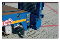
Support legs for extra stability during loading/unloading
